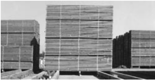
Figure 13–8. A sanitary, well-drained air-drying yard.
