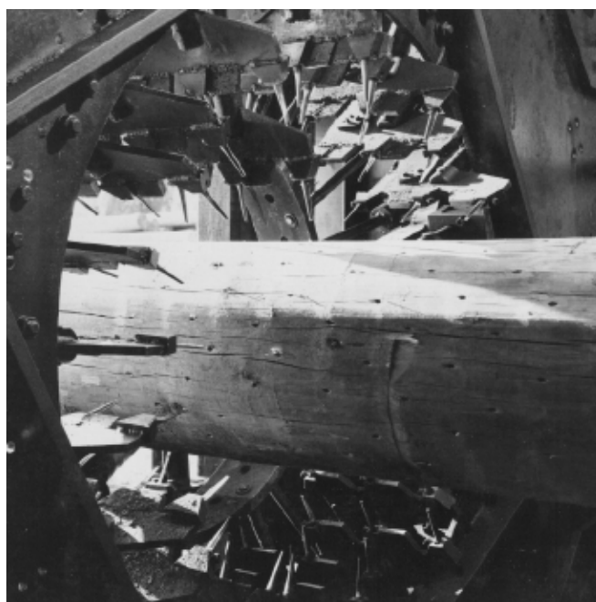
Figure 14-2. Deep incising permits better penetration of preservative.
