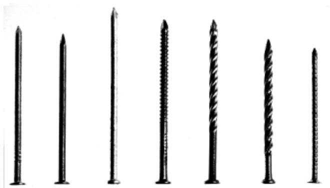
Figure 7-1. Various types of nails: (left to right) bright smooth wire nail, cement coated, zinc-coated, annularly threaded, helically threaded, helically threaded and barbed, and barbed.
