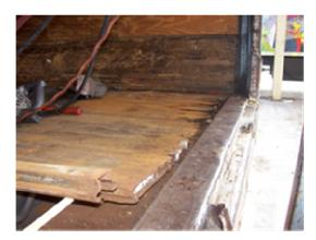
Prolam is offering a solution which consists of using a borate wood preservative that will prevent the fungus from occurring and will reduce the risk of decay. The wood preservative is locally applied to the area where the steel threshold plate will be installed. The treatment can be done during the manufacturing process of the laminated hardwood floor or the container, but always before the installation of the threshold steel plate.
